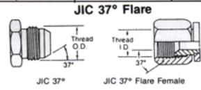
The JIC 37 degree flare male will mate with a JIC female only. The JIC male has straight threads and a 37 degree flare seat. The JIC female has straight threads and a 37 degree flare seat. The seal is made on the 37 degree flare seat. (Chart in next column)
