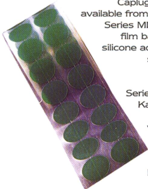
Caplugs Masking Discs are available from stock in two styles: Series MDG, a 2-Mil polyester film backing with a 1.5-Mil silicone adhesive that offers a superior resiliency at temperatures up to 400°F (204°C); and Series MDK, which has a Kapton® polyimide film backing that will withstand temperatures up to 500°F (260°C). Caplugs Masking Discs have broad applications in powder coating, electroplating, chrome plating, anodizing and solder wave applications.
